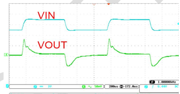
图 2 Line Transient (VIN=from 5.6V to 7V to 5.6V IOUT=150mA)
