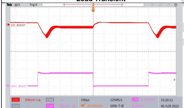
Boost, IOUT=0-150mA, 0.3A/us Load Transient
