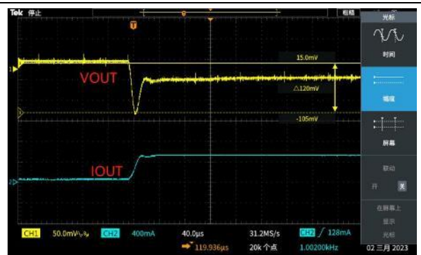
图 6 Load Transient ( V_{IN}=V_{OUT}+1V , I_{OUT}=500mA-50mA )
